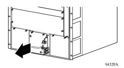
Lift the extractor lever to disconnect the power supply from the backplane connector.
